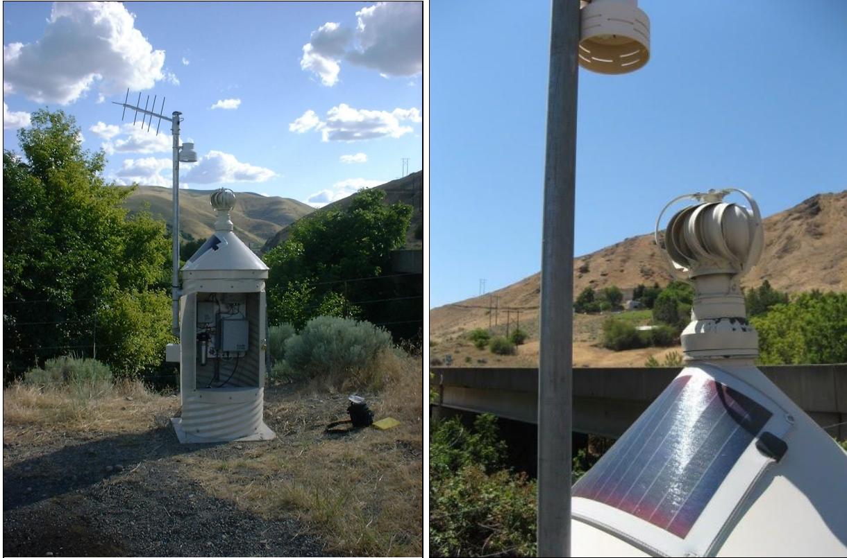
Figure 1. Washington State Department of Ecology weather station at Alpowa Creek, WA. The temperature sensor is located on the pole in the shielded unit above the metal instrument housing and solar panel.
