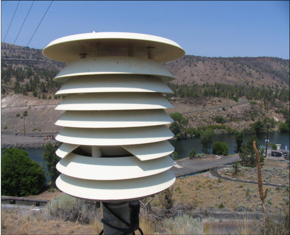
**Figure 13.** Photo of Pelton Dam COOP site MMTS showing the damaged fin.
