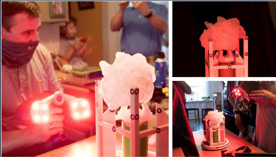
Figure 3: Photograph (left) of IBHS engineer Ross Maiden laser scanning the Hondo, TX hailstone, (top-right) photograph showing the laser plane tracking across the hailstone, and (bottom-right) the hailstone on the scanner mount. Photographs by Christina Gropp.
