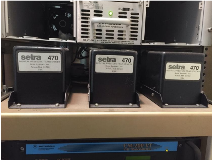
Figure 3: Photo of the pressure transducers at the Lamar airport, taken 7 May 2020, courtesy of Michael Nosko, NWS WFO Pueblo.
