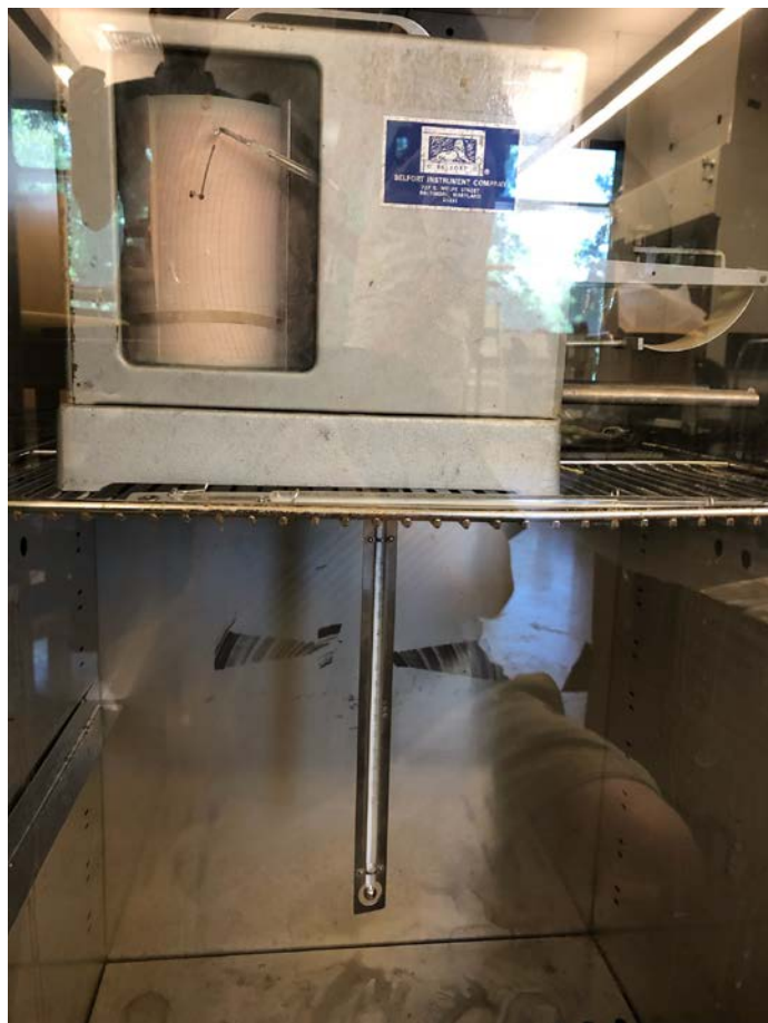
Fig. 5: Photo of the configuration of the thermometers in the oven, with the outer door open but the inner clear door closed. The thermograph is on the top rack and the LIG max-T thermometer is hanging below.
