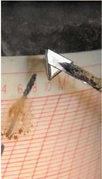
Fig. 8: Zoomed photo of thermograph while in the oven, showing the arm at the approximate maximum temperature.
