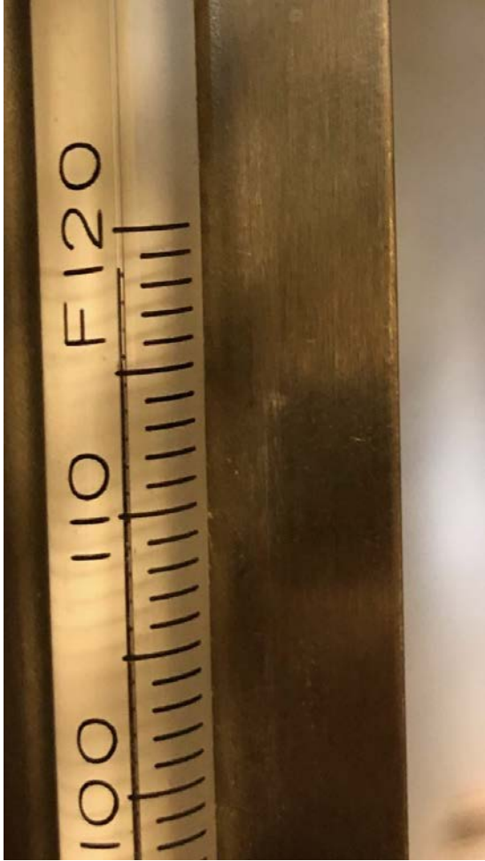
Fig. 6: Zoom-in on LIG thermometer showing a value of nearly 119°F after oven testing.
