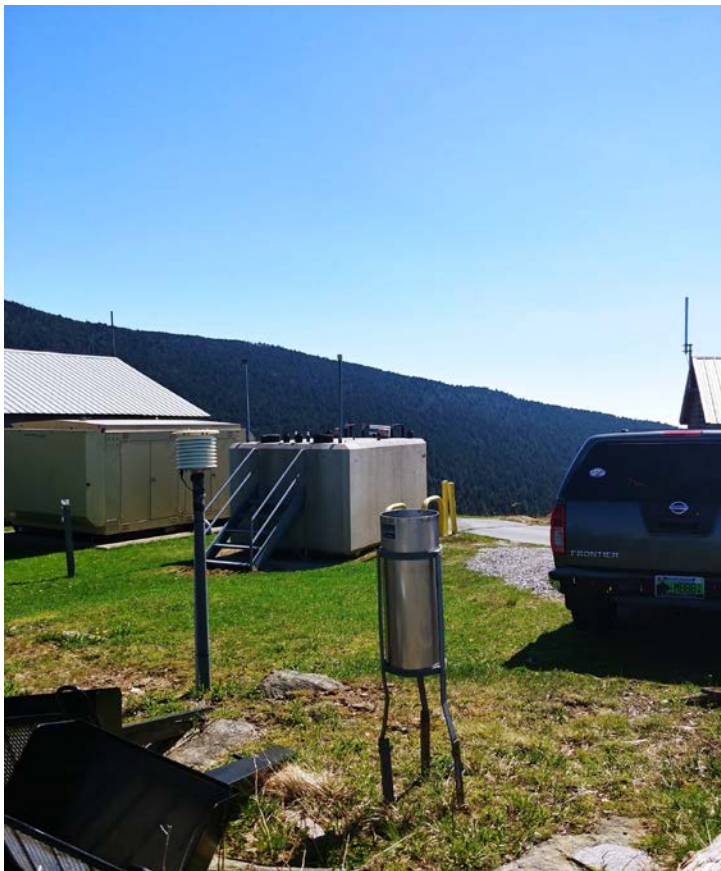
Figure 1. SRG, MMTS and Plastic rain gage. Courtesy of S.Heuser.
