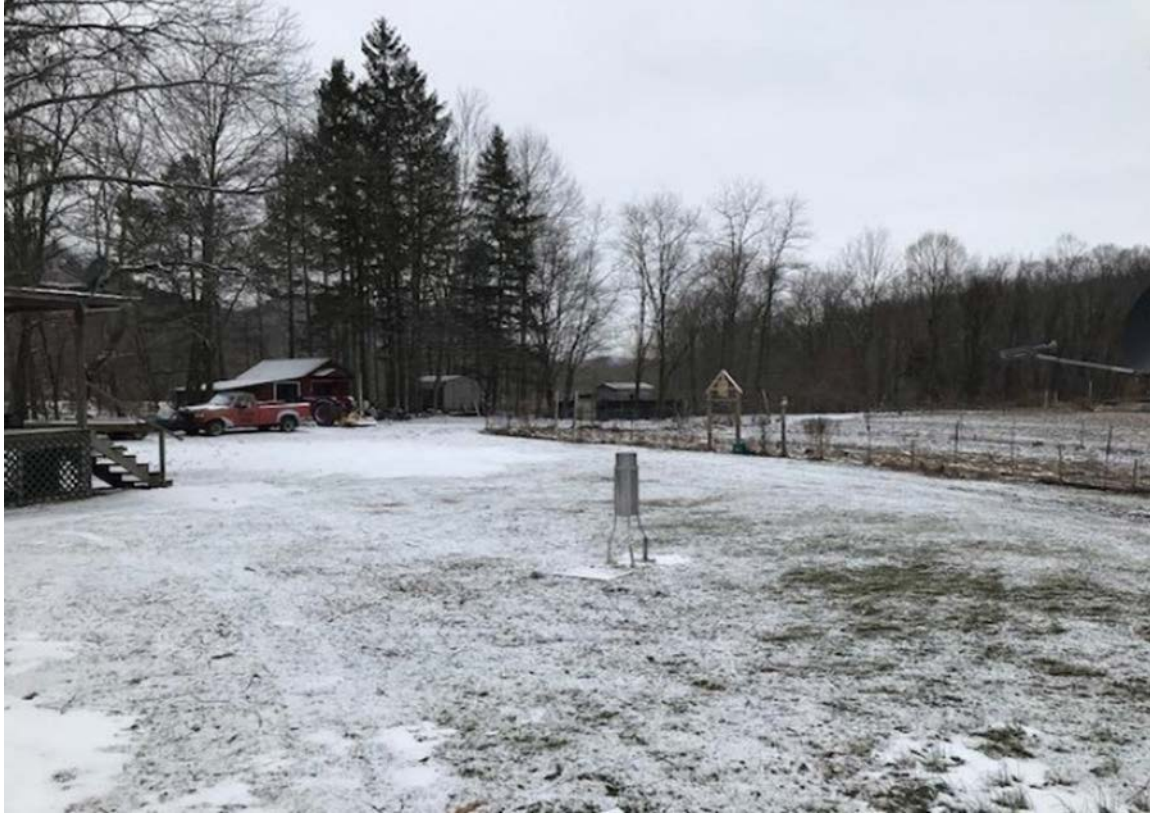
Fig. 2. View of standard 8 inch rain gauge located at Parsons 3SE, WV.
