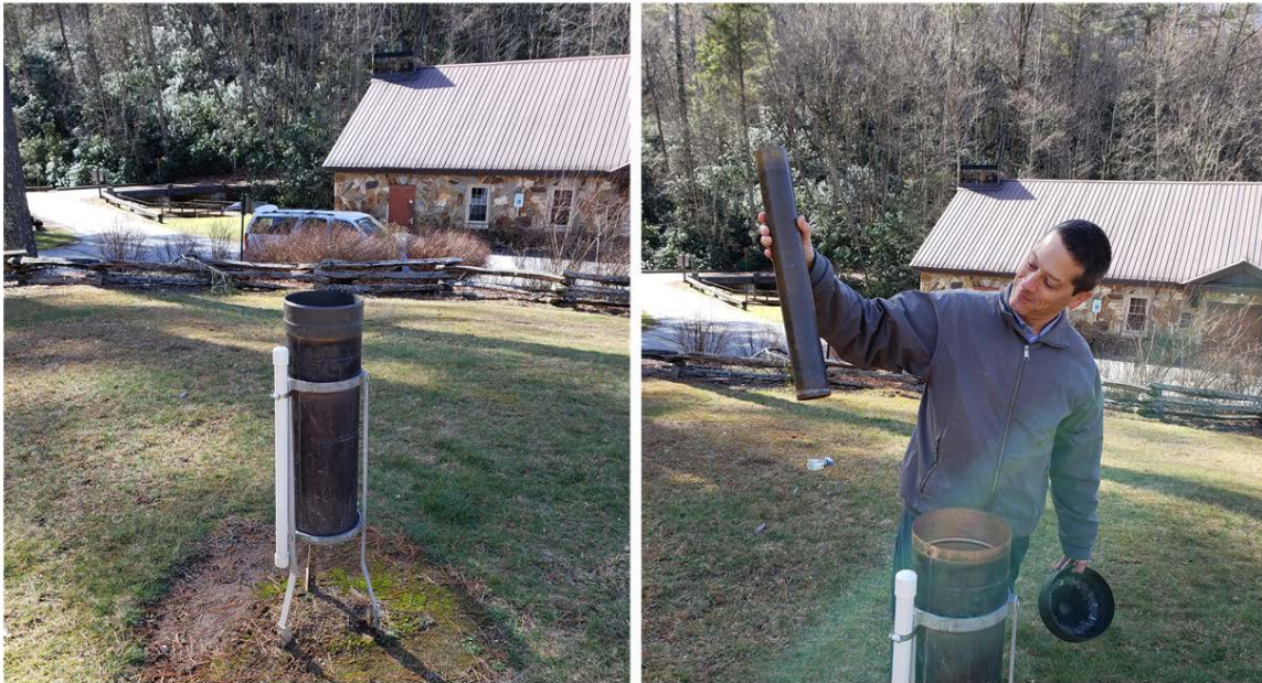
Figure 1. NWS Greenville-Spartanburg OPL Chris Horne inspecting the Jocassee SRG. Courtesy of M.Griffin.
