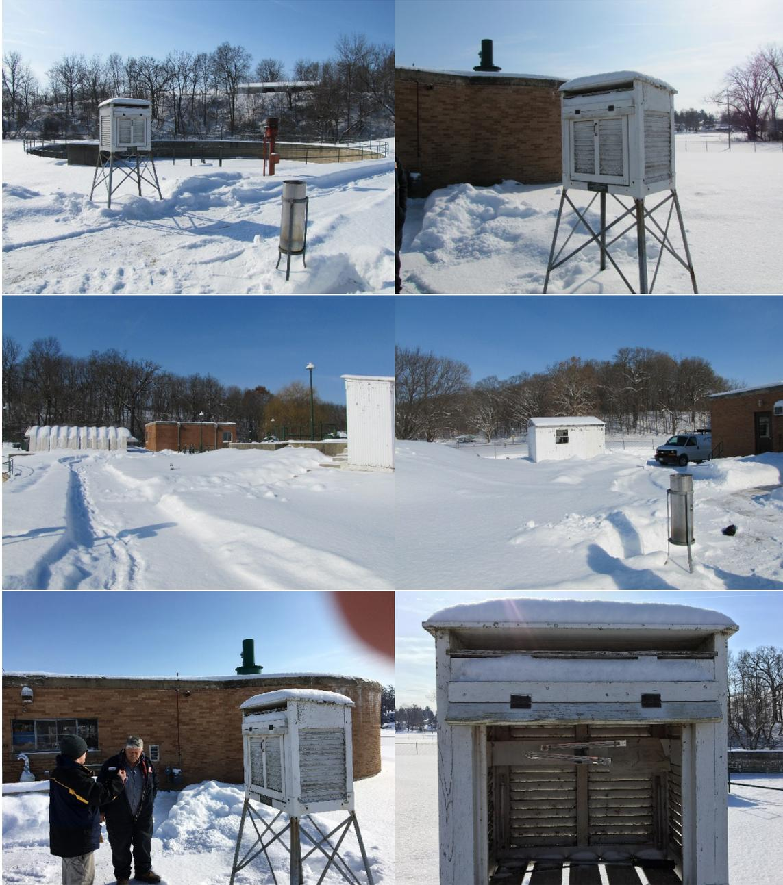
Figure A3. Instrumentation is a standard Cotton Region shelter with two glass thermometers, alcohol in glass for minimum temperatures and mercury in glass for maximum temperatures. Bill Zink, plant superintendent, was the observer and has been serving for one year. The time of observation was 7:15 am CST. (Photos: Quad Cities WFO)
