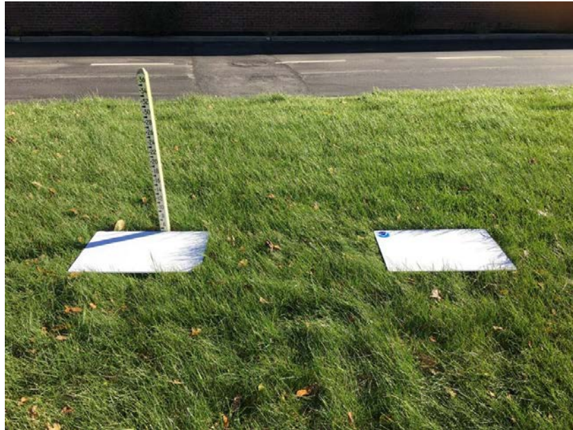
Figure 3. Snowfall and snow depth boards located at Erie Airport.
