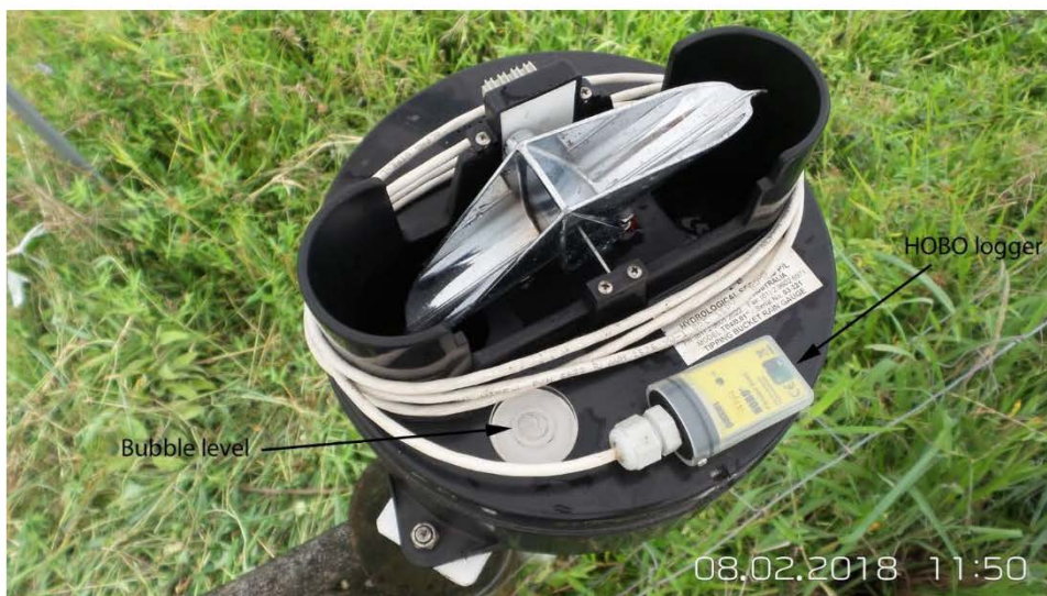
Figure 2. Close up of tipping buckets in operational configuration. Note bubble level indicates gage is slightly tilted.
