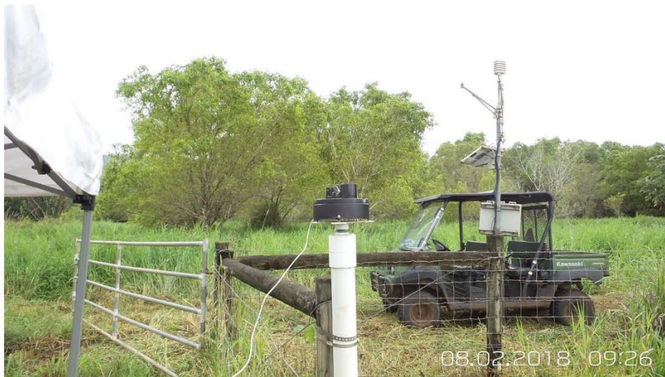
Figure 1. View of Waipa Garden tipping bucket rain gage mounted on PVC post. Enclosure has been removed in the image. Java plum trees are in the background and do not interfere with rainfall catch.
